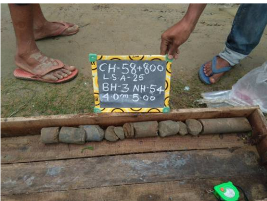
PICTURE 221: BH-3 (Depth-4.00m to 5.00m)
